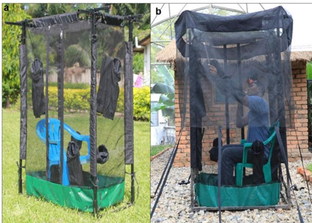
Fig. 2 Miniaturized Double Net Trap (DN-Mini). A Provides a clear picture of DN-Mini trap and B show a volunteer collecting mosquito while seating down but not freely exposed to mosquitoes
