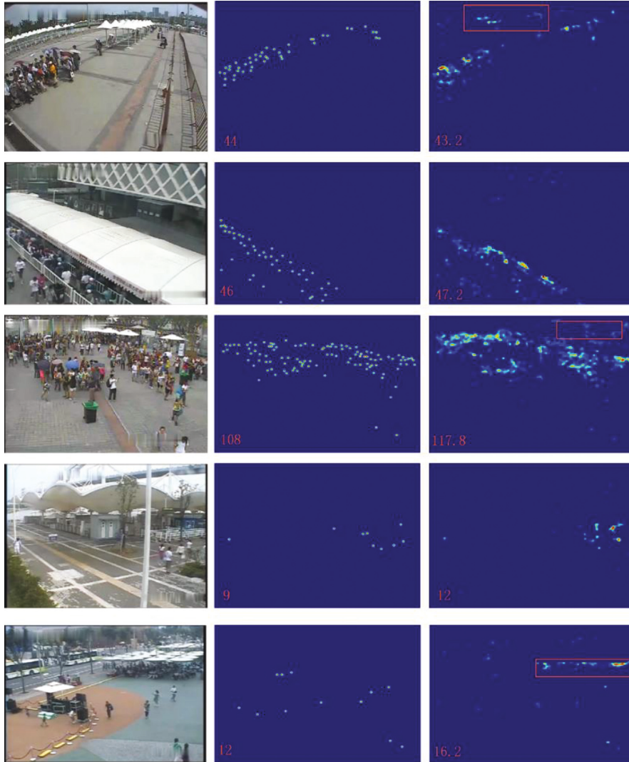
FIGURE 8: Comparison of visual results on WorldExpo'10. The first, second, and third columns show test samples, the corresponding ground truth, and the generated density map, respectively. The box outlined in red represents the area where we mistook the background for a head.
