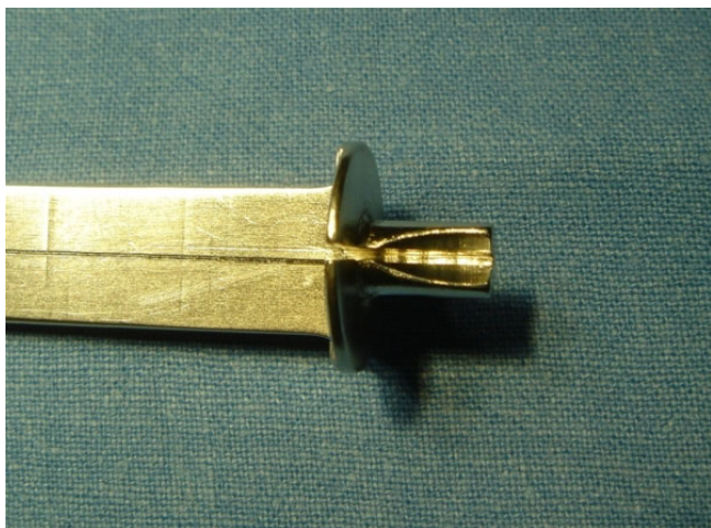
Figure 13 Object 6. The slit is still too large and it cannot be used in off-pump patients.
