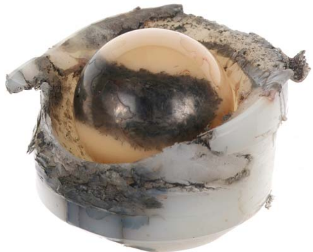
Fig. 6 Erosion of the polyethylene liner and resulting metallosis and staining
