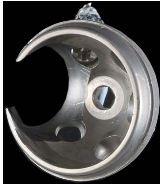
Fig. 2 The ceramic femoral head had eroded through the polyethylene liner and metal acetabular component. The heads of the cancellous fixation screws were also worn
