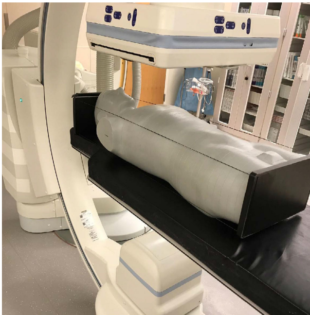
FIG. 2. Anthropomorphic phantom experiment setup using 12 radiation events with different kVp, Cu filter, field size, and angle. Dose to air was measured under the torso of the phantom with a Radcal 10x6-0.6 ion chamber, and corrected using B_{PMMA}^{st} . The measured surface dose was compared to results predicted by Eqs 7–9 and Eq 1. Results are shown in Table 6. PMMA, polymethyl methacrylate.
