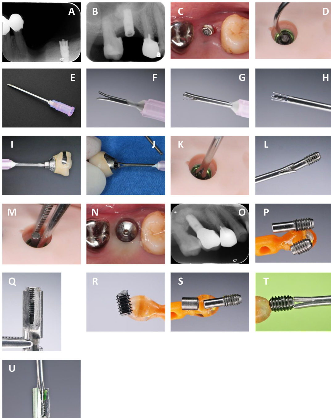
Figure. 1 Clinical intraoral photographs and radiographs of our cases and clinical simulations. (A) The level of screw fracture was above implant platform. (Zimmer Dental, TSV® Dental Implant 4.5mmD; Palm Beach Gardens, FL, USA) (B) The level of screw fracture was deep in the implant. (Nobel Biocare, Branemark Implant WP, Zurich, Switzerland). (C) Implant platform and abutment screw fragment were partially covered by the gingiva. (Nobel Biocare, Branemark Implant WP) (D) The screw fragment was pushed by the #TU23-end of the dental explorer to verify the mobility of the screw fragment. (E, F, G and H) Two-, three- and four-claw custom-made screwdriver were modified from an 18-gauge syringe needle. (I and J) Adjust the claws to be slightly larger than the fractured screw. (K) The claws grasped the fractured screw. (L and M) The screw fragment removed by the custom-made screwdriver or by mosquito forceps. (N) The new healing abutment in place. (O) After adjusting the overhanging restoration of tooth 17, the old crown with a new abutment screw was delivered. (P) Abutment screw fracture occurred at the different levels. (Q) Sectioned implant replica; note the gap between the abutment screw and the inner thread of the implant replica. (Nobel Biocare, Branemark Implant RP). (R) A small protuberance at the fractured surface of the abutment screw. (S) The horizontal fractured surface was relatively flat with no protuberance (Zimmer Dental, TSV® Dental Implant 4.5mmD). (T) Multiple contact points between the claws and the fractured screw surface. (U) The claws of a custom-made screwdriver grasped the fragment of the fractured screw.
