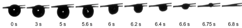
Fig. 3. Shadowgraph images extracted from a video of the combustion of a diesel-butanol droplet.
