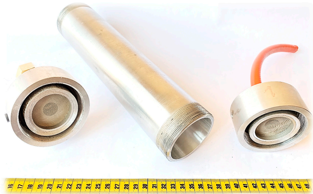
Figure 3. Aluminum pipe used in the experiment as a container for disintegrated rock.
