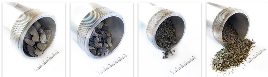
Figure 4. Rock material prepared for the experiment, in four different grain size classes.
