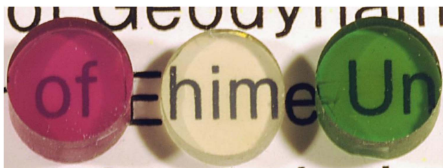
Figure 6 | Transparent nano-polycrystalline garnets with various chemical compositions. Some examples of high-quality polycrystalline garnet synthesized at 15 GPa and at 1,400 °C, with a diameter of ~4 mm and thickness of ~2 mm; grossular with 2 mol% \text{Ca}_3\text{Cr}_2\text{Si}_3\text{O}_{12} uvarovite (green), pure grossular (colourless) and \text{Mg}_3\text{Al}_2\text{Si}_3\text{O}_{12} pyrope with 5 mol% knorringite \text{Mg}_3\text{Cr}_2\text{Si}_3\text{O}_{12} (purple).
