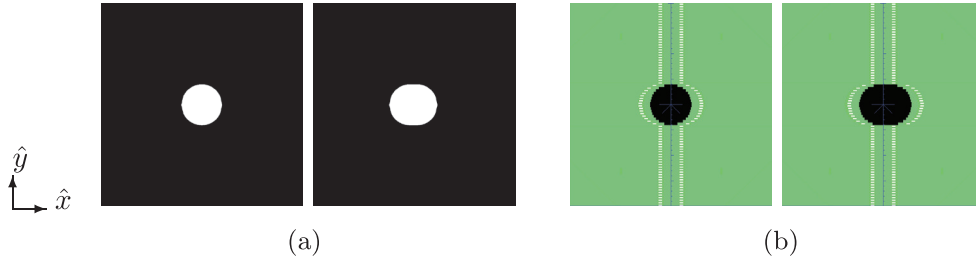
Figure 3. (a) shows the effect of margin-controlled dilation on rasterized polygons; the original aperture (left) is dilated in \hat{x} -direction. From the contours of the dilated shape, a new valid MLC-segment is calculated by the leaf-shaping algorithm (b). (a) Rasterized polygon segments. (b) Prescribed segments.
