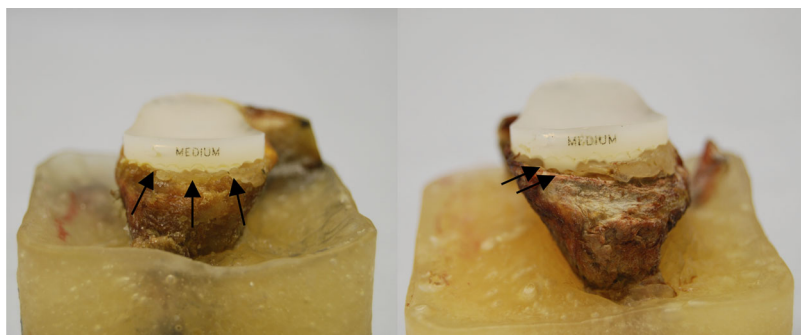
Figure 3. Failure definition: “partial failure” as inferior rim distracts away from cement (left) and “failure” as inferior pegs visible (right).
