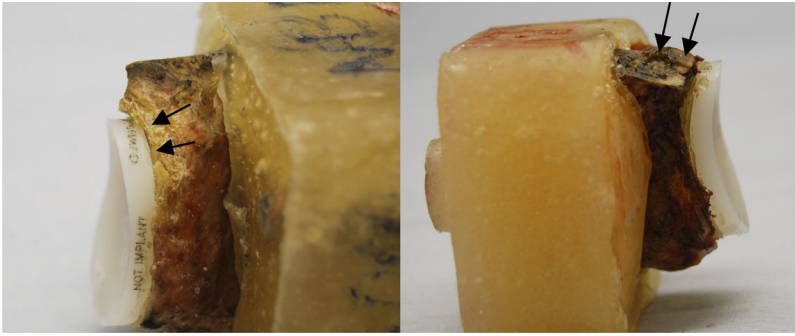
Figure 4. Superior failure-rim distracts away from cement (left) and bone crushing-bone fracture or implant embedding (right).
