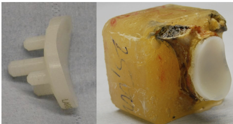
Figure 1. Curved-back cemented glenoid implant (left). Cadaveric scapula cemented and potted for testing (right).
