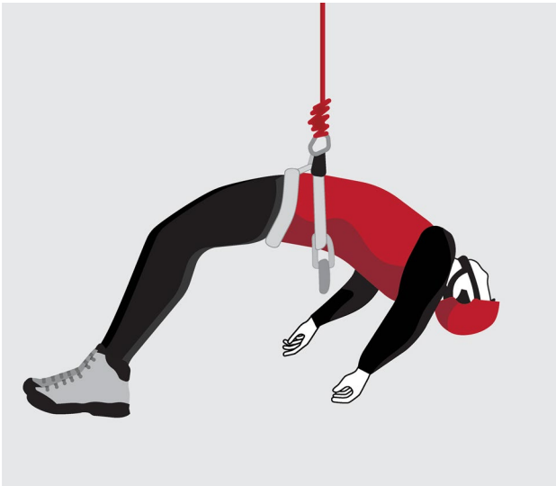
Fig. 5 In an unconscious person suspended in a sit harness, the attachment point of the rope, located at the level of the hips will represent the highest point
