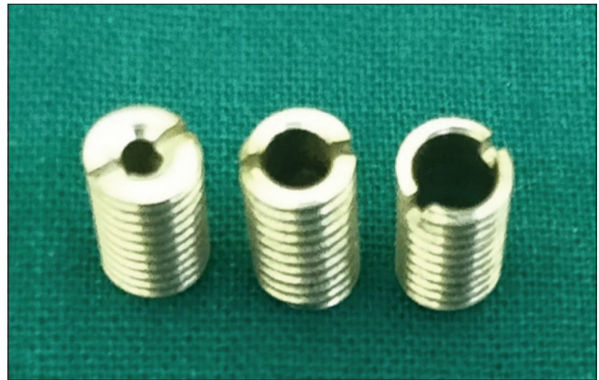
Figure 2: Drill bit guide with different internal diameters (2.1, 3.6, and 4.4 mm) of inner rings
