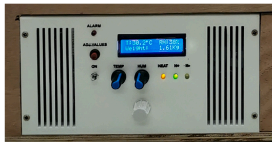
Fig. 9. Frontal wall of the electronics drawer without pressing the pushbutton.
