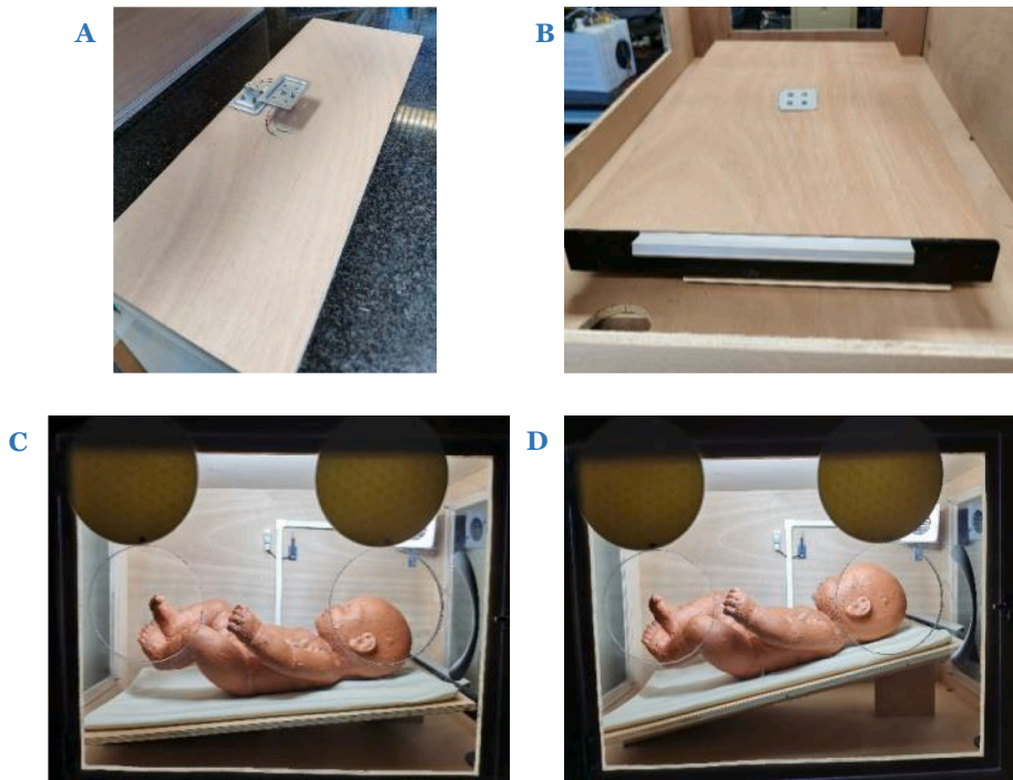
Fig. 3. (A) Weight sensor placement. (B) PLA structure with the handle. Inclination of the bed 6° (C) and 12° (D) by using the wooden wedges.
