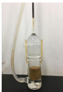
Figure 2. Modified Amott cell used for imbibition tests.
