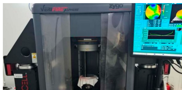
Figure 3. Six-inch aspheric vertical interferometer of Zygo VerFire Asphere.
