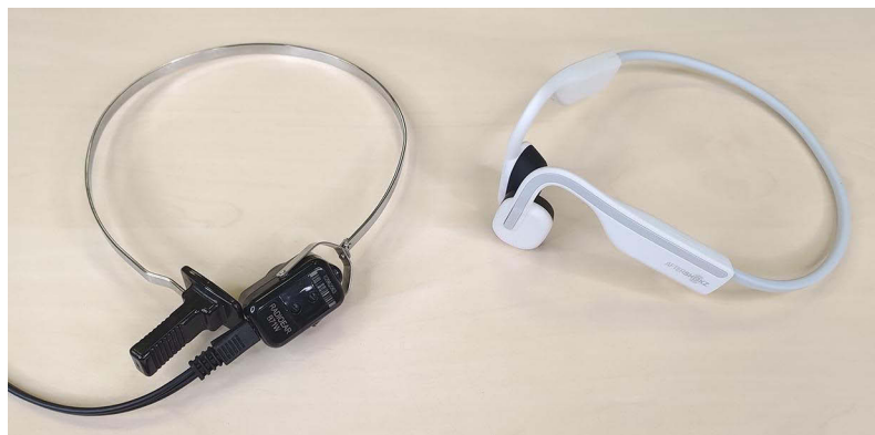
Figure 4 B71 bone transducer (left) and AfterShokz OpenMove open-ear headphones (right). Reprinted from Masalski M, Turski M, Zatoński T. Self-assessment of bone conduction hearing threshold using mobile audiometry: comparison with pure tone audiometry. Int J Audiol. 2023;1-8. Creative Commons. 13
