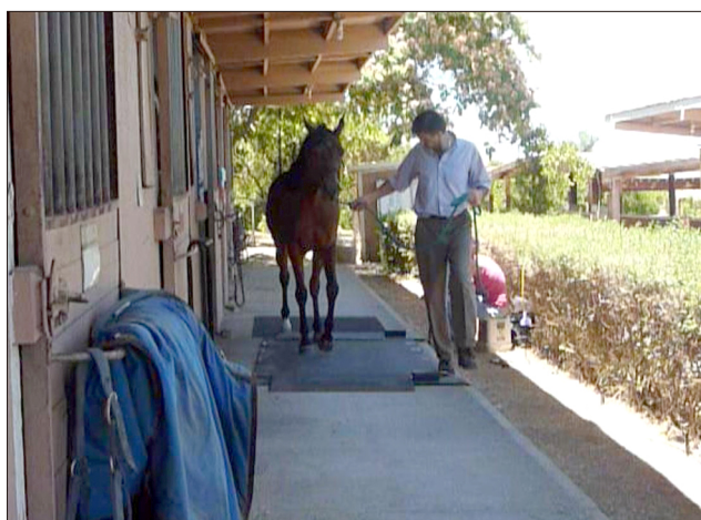
Fig. 1. A horse being walked on the pressure plate during a preliminary trial. The plate is covered with a thin rubber mat for plate protection and is connected to a laptop to collect data.
