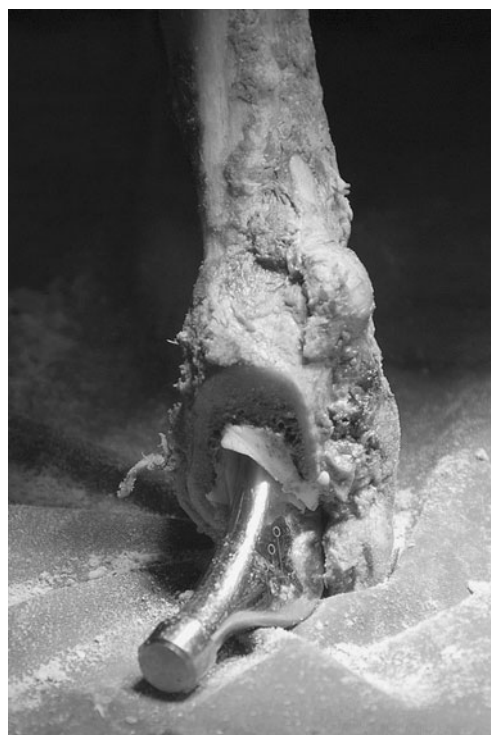
Fig. 3 The removable Exeter prosthesis is shown partly dislodged from one of the test femora
