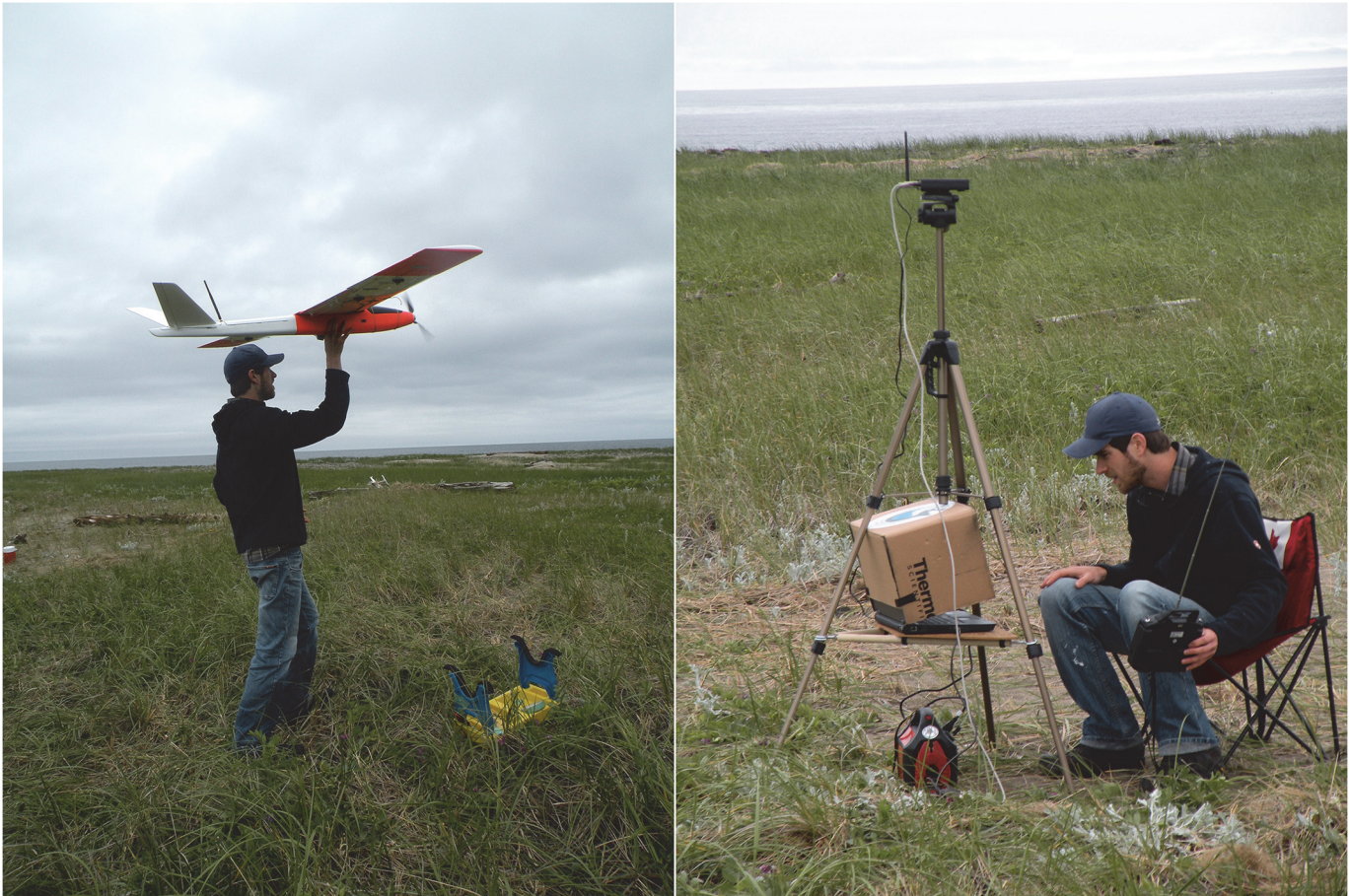
Fig 3. The AI-Multi electric unmanned aircraft and ground control station. Shown on the left prior to hand-launch from the South Kouchibouguac Dune, Kouchibouguac National Park, New Brunswick, 2012. The ground control station is composed of a laptop and radio modem mounted on a modified camera tripod, as well as a portable power supply.
