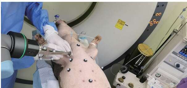
Figure 6 An operator uses this robot-assisted puncture system for biopsy in an experimental pig.
