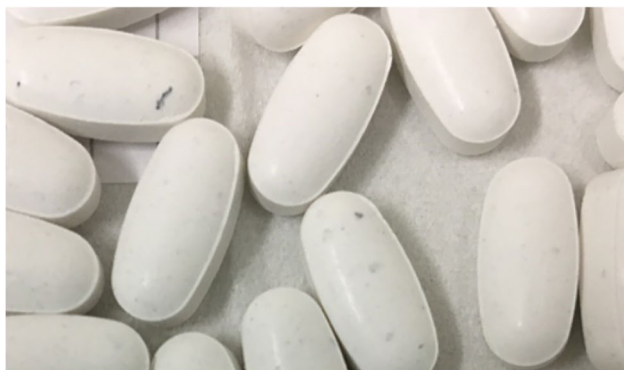
Fig. 4 Tablets with visual defects caused by abrasion effects during twin screw wet granulation process
