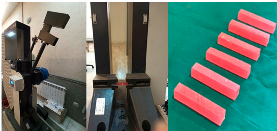
Figure 4. Pendulum Charpy impact testing machine and prepared specimens.
