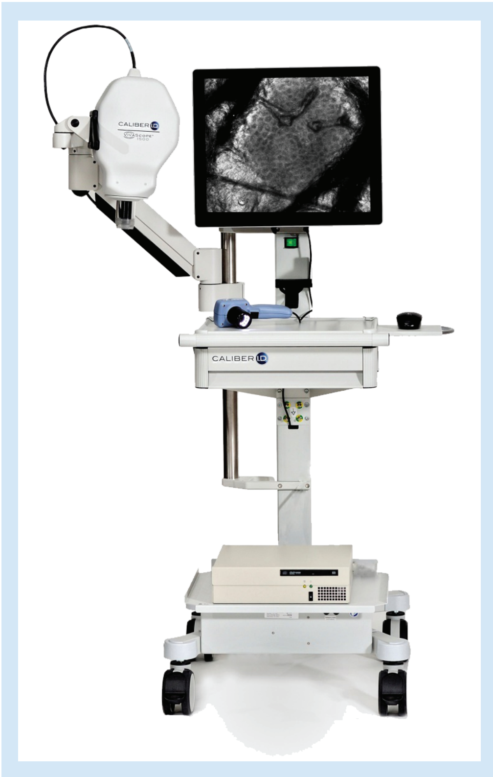
Figure 2. Vivascope® 1500: the microscope is coupled to a dermatoscope. Prior to imaging, the large probe must be fixed to the patient's skin. Reproduced with permission from Caliber Imaging & Diagnostics, Inc., NY, USA.
