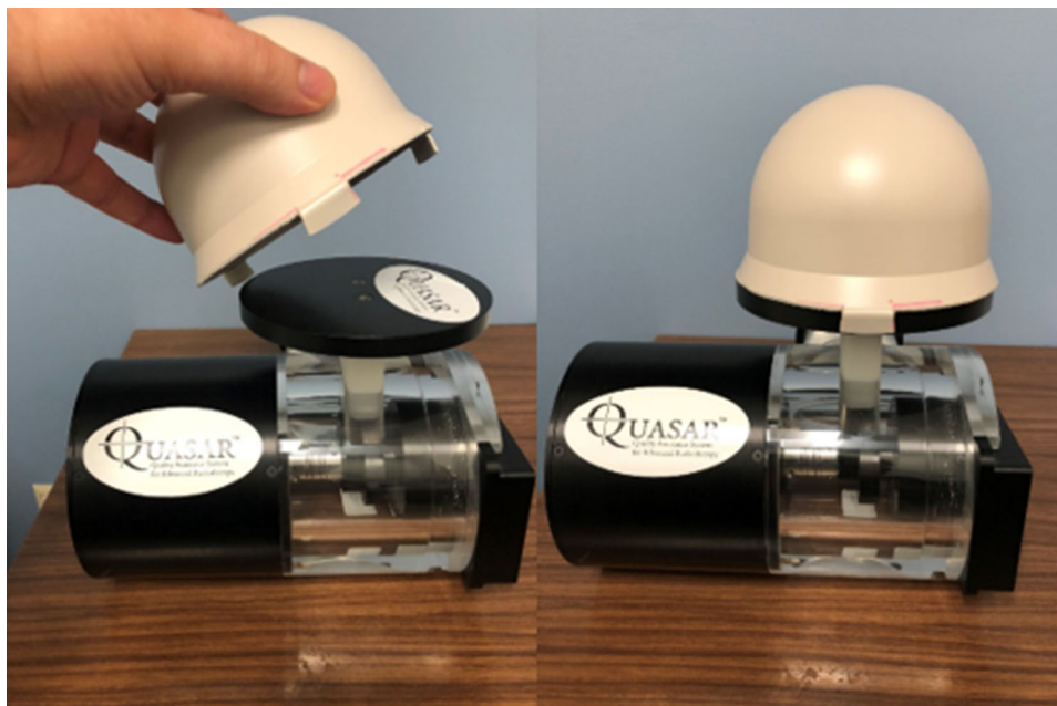
FIGURE 5 A home-made breast phantom (in beige) can be attached to the flat chest wall phantom (in black) for enhanced surface tracking of respiratory motion.
