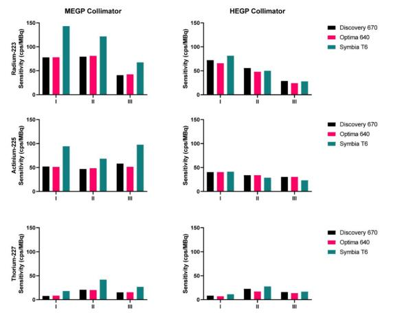
**Figure 4.** Sensitivities measured on the three gamma cameras with both collimators, for the three isotopes:  $^{223}$ Ra (top),  $^{225}$ Ac (middle),  $^{227}$ Th (bottom). The energy windows I, II and III are: 85 keV ± 20%, 154 keV ± 20%, and 270 keV ± 10% for  $^{223}$ Ra; 82 keV ± 20%, 216.8 keV ± 8%, and 444.3 keV ± 5% for  $^{225}$ Ac; 50.6 keV ± 20%, 85.7 keV ± 15%, and 240 keV ± 9% for  $^{227}$ Th.
