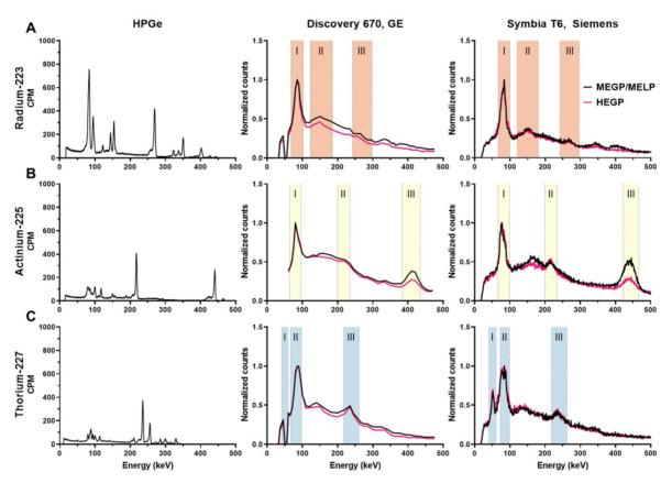
Figure 3. High resolution and clinical imaging system derived energy spectra of: A) <sup>223</sup>Ra, B) <sup>225</sup>Ac, C) <sup>227</sup>Th. Left column: energy spectra measured by HPGe. Middle column: energy spectra measured on the Discovery 670 (GE) with the MEGP and HEGP collimators. Right column: energy spectra measured on the Symbia T6 (Siemens) with the MELP and HEGP collimators. The shaded areas are the chosen emission energy windows for SPECT evaluation.
