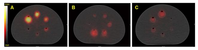
Figure 5. SPECT/CT fusion of the NEMA phantom acquired on the Discovery 670 (GE) with the HEGP collimator. Images are of A) Spheres filled with 40 kBq/mL of <sup>223</sup>Ra; B) spheres filled with 35 kBq/mL of <sup>225</sup>Ac, C) spheres filled with 40 kBq/mL of <sup>227</sup>Th.
