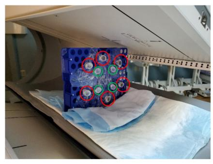
**Figure 2.** Limit of detection phantom scanned by the Optima 640 gamma-camera. The six identical conical polypropylene vials are filled with different concentrations of <sup>223</sup>Ra: 74, 37, 27.7, 18.5, 9.2, and 3.7 kBq/mL. The red circles denote the vials containing the hot sources while the green circles denote the vials filled with water.
