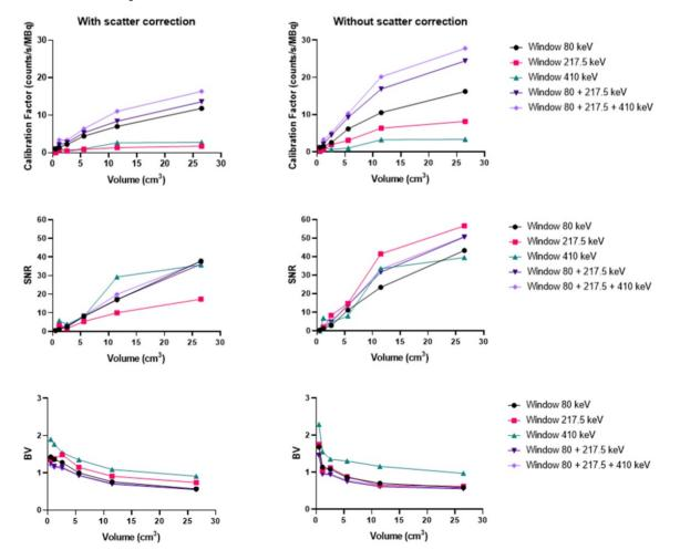
Figure 9. Calibration factors, SNR and BV measured on SPECT/CT images of the NEMA phantom filled with <sup>225</sup>Ac for each energy window and combination of energy windows. The images were acquired on the Optima 640 (GE) with the HEGP collimator with scatter correction (left column) and without (right column).
