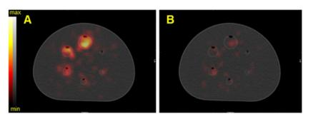
Figure 7. SPECT/CT fusion of the NEMA phantom acquired on the Optima 640 (GE) with the MEGP collimator. The phantom spheres were filled with 35 kBq/mL of <sup>225</sup>Ac. A) Reconstructed image of the 217.5 keV ± 8% emission window without scatter correction, B) Reconstructed image of the 217.5 keV ± 8% emission window with scatter correction.
