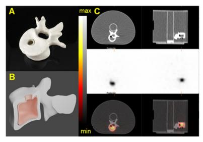
**Figure 13.** 3D-printed Vertebrae phantom. A) Picture of a 3D printed Vertebrae. B) CAD of the Vertebrae showing the fillable space. C) The Vertebrae phantom was fixed on the cylindrical insert inside the NEMA phantom SPECT/CT images of the 3D-printed vertebrae phantom acquired on the Discovery 670 with the MEGP collimator. Transaxial and Sagittal views of the Vertebrae phantom filled with 40 kBg/mL of <sup>223</sup>Ra. Top: CT view. Middle: NM view. Bottom: NM/CT fusion.
