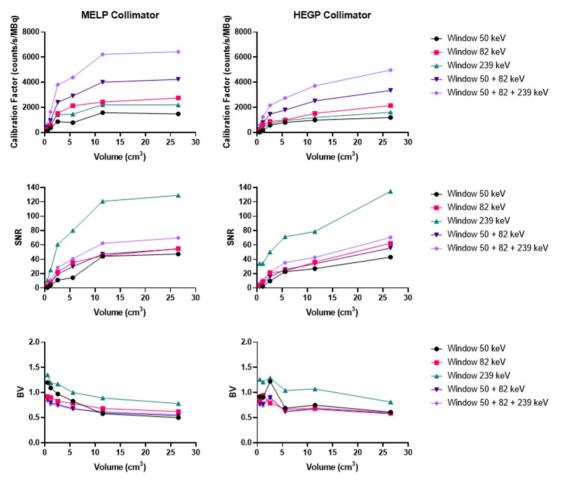
Figure 10. Calibration factors, SNR and BV measured on SPECT/CT images of the NEMA phantom filled with <sup>227</sup>Th for each energy window and combination of energy windows. The representative data were acquired on the Symbia T6 (Siemens) with the MELP (left column) and HEGP (right column) collimators.
