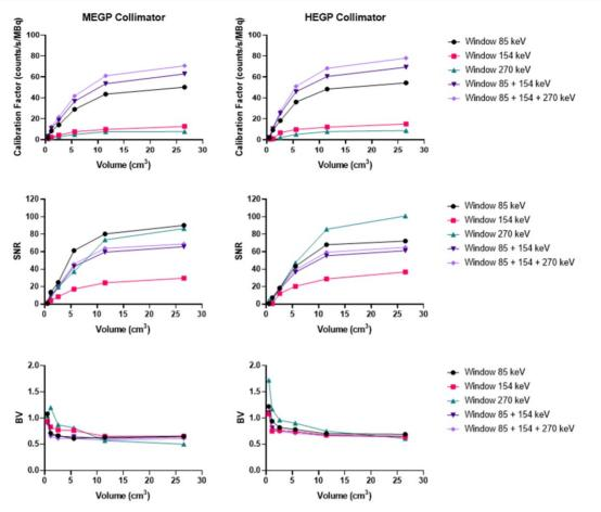
Figure 8. Calibration factors, SNR and BV measured on SPECT/CT images of the NEMA phantom filled with <sup>223</sup>Ra for each energy window and combination of the energy windows. Representative data acquired on the Discovery 670 (GE) with the MEGP (left column) and HEGP (right column) collimators.
