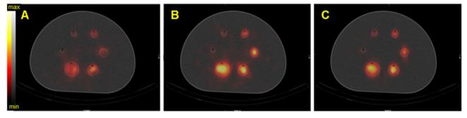
Figure 6. SPECT/CT fusion of the NEMA phantom acquired on the Symbia T6 (Siemens) with the MELP collimator. The phantom was filled with 40 kBq/mL of  $^{227}$ Th. A) Reconstructed image of the 50.6 keV  $\pm$  20% emission window, B) reconstructed image of the 85.7 keV  $\pm$  15% emission window, C) reconstructed image of the 240 keV  $\pm$  9% emission window.
