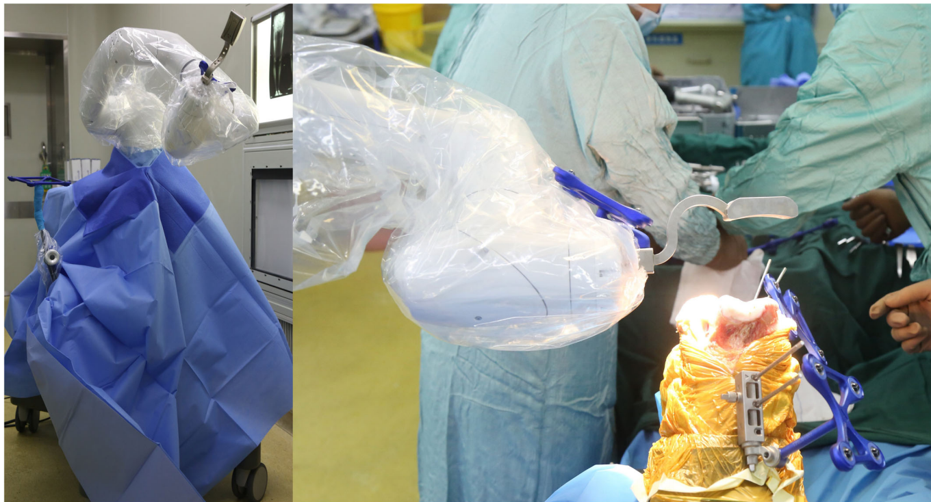
Fig. 1 Innovative design of the SkyWalker™ robotic arm system. The SkyWalker™ robotic arm consists of six joints, with a wide range of motion and flexible operation. The cutting jig is stably connected to the end of the robotic arm. An eccentric shaft is added to the cutting jig, which enables the latter to avoid the patella and patellar tendon to reduce osteotomy errors
