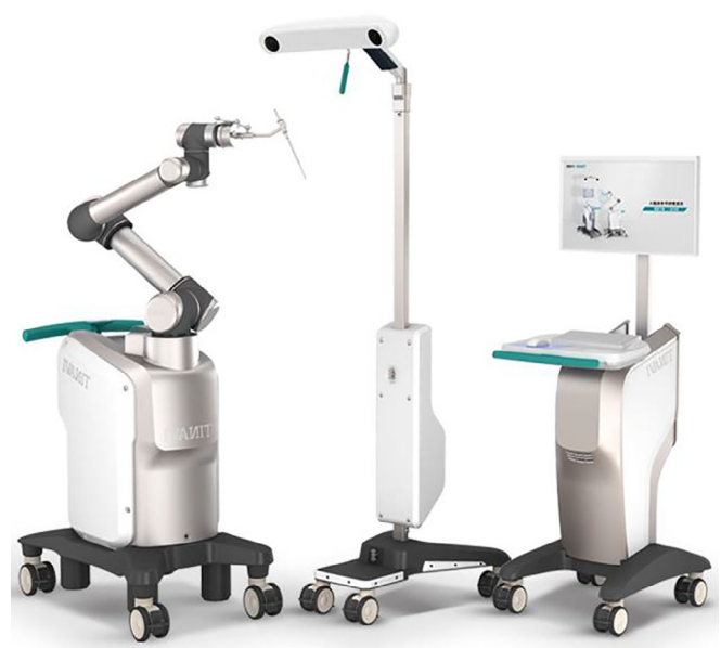
Fig. 1 TiRobot, mainly composed of a workstation, an optical tracking system, and a robotic arm (Photo provided by Beijing Tianzhihang Medical Technology).
