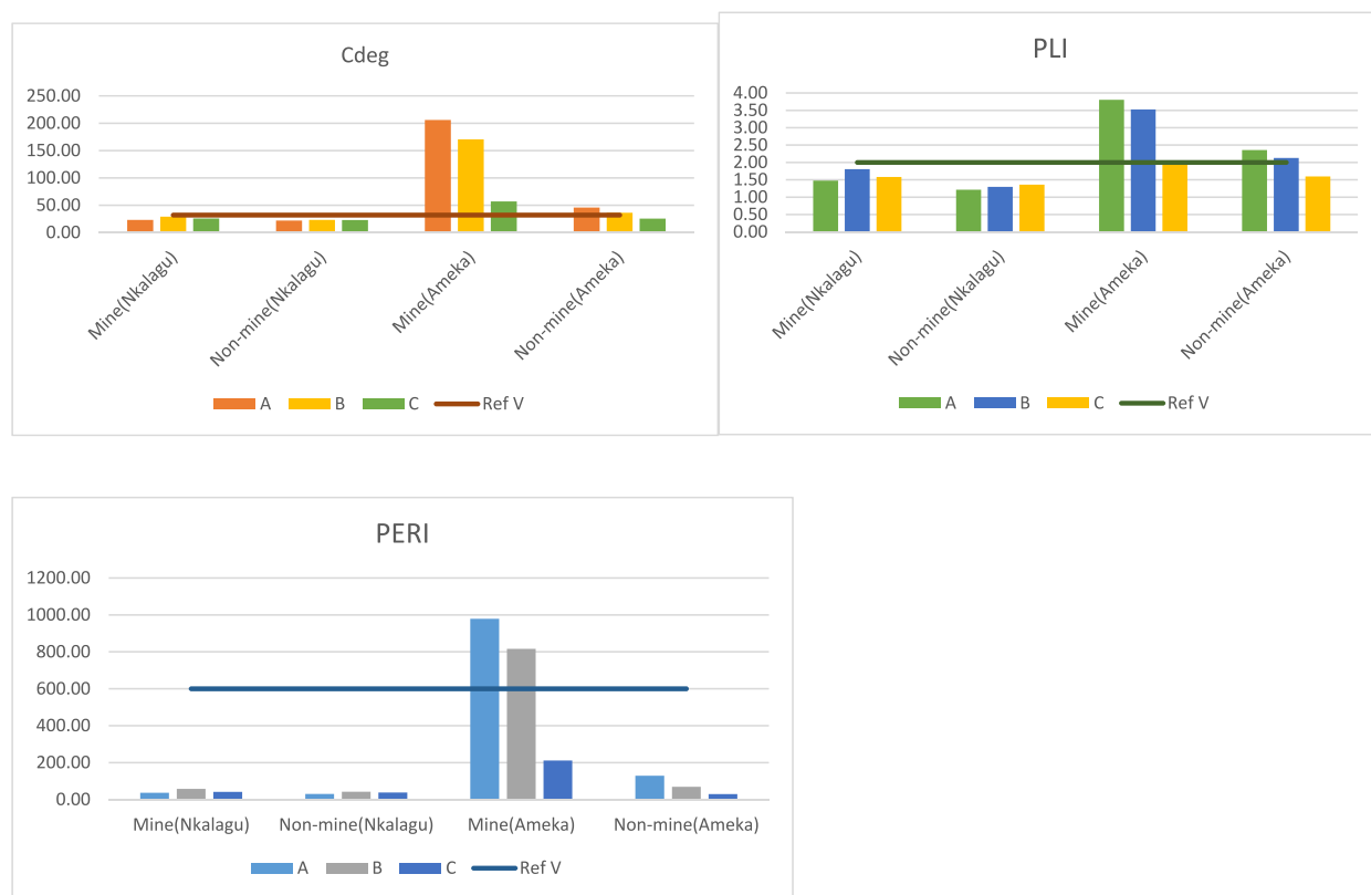
Fig. 8. Mean soil pollution load index, degree of contamination and potential ecological risk index for PTE in the studied soil.
