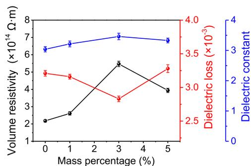
**Figure 6.** Volume resistivity (black line), dielectric constant (blue line), and dielectric loss (red line) of *m*-ABA-SiO<sub>2</sub>/CE nanocomposites with different mass percentages.
