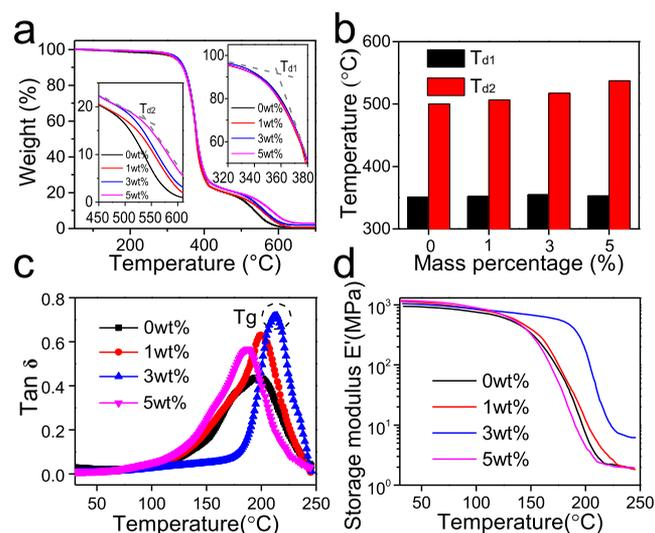
**Figure 4.** Effect of different mass fractions on the thermal stability of *m*-ABA-SiO<sub>2</sub>/CE nanocomposites. (a) TG curve; (b) distribution of the decomposition temperature ( $T_d$ ) histogram; (c) DMA curve; and (d) variation curve of the storage modulus between 20 and 250 °C.
