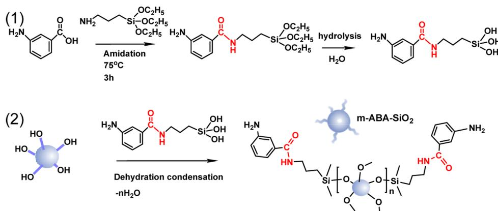
**Figure 2.** Diagram of the preparation mechanism of  $m\text{-ABA-SiO}_2$ . (1)  $m\text{-ABA}$  is connected to KH-550 through the amidation reaction and hydrolysis is completed. (2)  $\text{Si-OH}$  on  $m\text{-ABA-KH-550}$  and  $\text{SiO}_2$  are dehydrated and condensed to form  $\text{Si-O-Si}$  bonds to prepare  $m\text{-ABA-SiO}_2$ .
