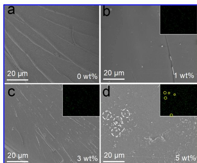
**Figure 3.** SEM images of the cross section of the *m*-ABA-SiO<sub>2</sub>/CE nanocomposite material. (a–d) CE-based nanocomposites doped with (0, 1, 3, and 5 wt %) *m*-ABA-SiO<sub>2</sub> nanoparticles. The inset pictures (b–d) are Si element mapping in CE-based nanocomposites doped with 1, 3, and 5 wt % *m*-ABA-SiO<sub>2</sub> nanoparticles, respectively.
