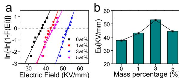
**Figure 7.** Electrical breakdown performance of *m*-ABA-SiO<sub>2</sub>/CE nanocomposites. (a) Weibull distribution of measured breakdown strengths of nanocomposites. The solid lines refer to the fitting results using a two-parameter Weibull distribution function (see the Experimental Section). (b) Effect of *m*-ABA-SiO<sub>2</sub> with different mass percentages on CE-based nanocomposites' breakdown field strength ( $E_b$ ).
