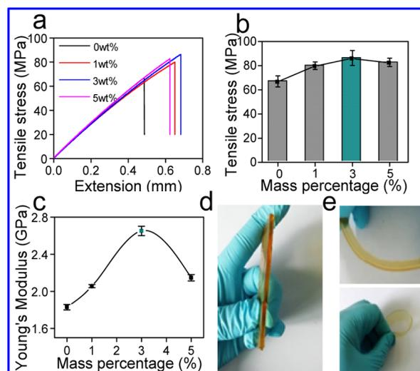
**Figure 5.** Influence of different mass fractions on the mechanical properties of *m*-ABA-SiO<sub>2</sub>/CE nanocomposites. (a) Stress–strain curve; (b) distribution of the tensile strength histogram; (c) Young's modulus curve; (d) brittleness of pure CE; and (e) *m*-ABA-SiO<sub>2</sub>/CE nanocomposite material's certain flexibility.
