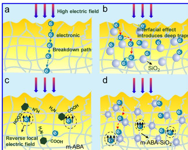
**Figure 1.** Diagram of the breakdown schematic of electrons on different bases. (a) Electrical breakdown schematic of pure CE; (b) electrical breakdown schematic of the  $\text{SiO}_2/\text{CE}$  nanocomposite; (c) electrical breakdown schematic of the  $m\text{-ABA}/\text{CE}$  composite; and (d) electrical breakdown schematic of the  $m\text{-ABA-SiO}_2/\text{CE}$  nanocomposite.
