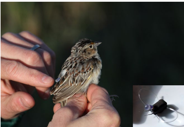
FIGURE 1 A Grasshopper Sparrow wearing a geolocator (stalk visible at fingertip) prior to release at Camp Grafton, ND, May 2015. The communication wires (for turning on the unit via a laptop software connection) on the geolocator (inset) were trimmed prior to deployment. Photographs by Alex Lehner and Inez Hein (inset)
