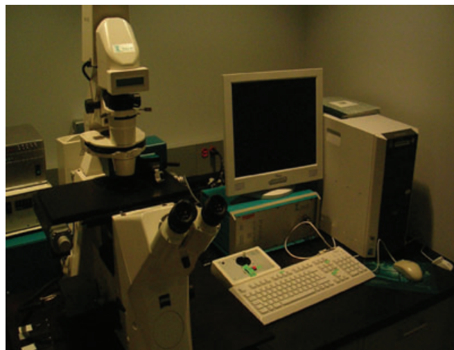
Figure 7. The Zeiss PALM apparatus. This instrument is used for the laser cutting (catapulting) procedure and requires a room with ample moisture so that random static discharges do not interfere with sample collection.
