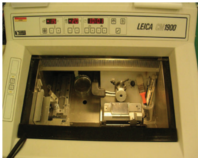
Figure 3. The Leica CM1900 Cryostat. This apparatus is used to section frozen tissue onto slides.
