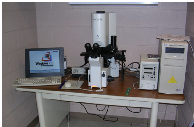
Figure 8. The Arcturus PixCell Iie apparatus. This instrument is used for the laser capture procedure and requires a room with low moisture so that tissues remain amply dry during cell collections.
