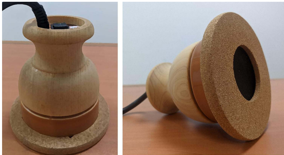
Figure 3 Electronic moxibustion device with its insulating material.
