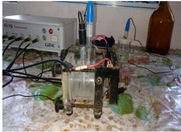
Fig. 10. Actual experimental setup for Potentio dynamic polarization.
