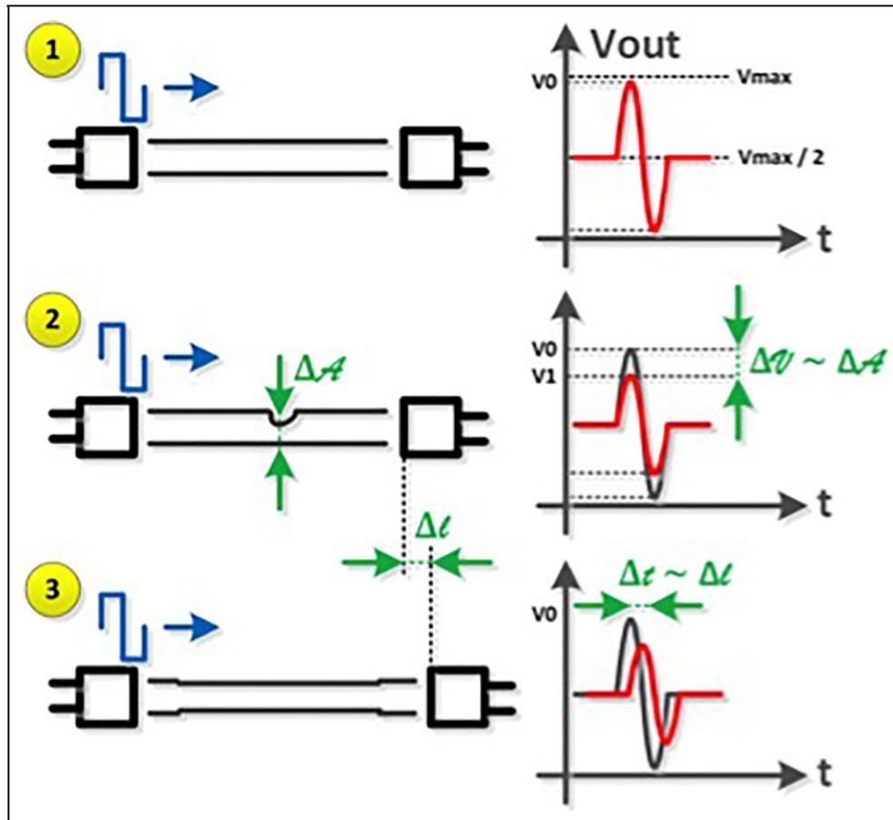
**Figure 2.** The signal in (1) is the normal signal of a non-touched nerve root. In (2) the analysis of the nerve contusion (measurement of absorption) and in (3) the nerve tension (measurement of the time shift) is shown.
