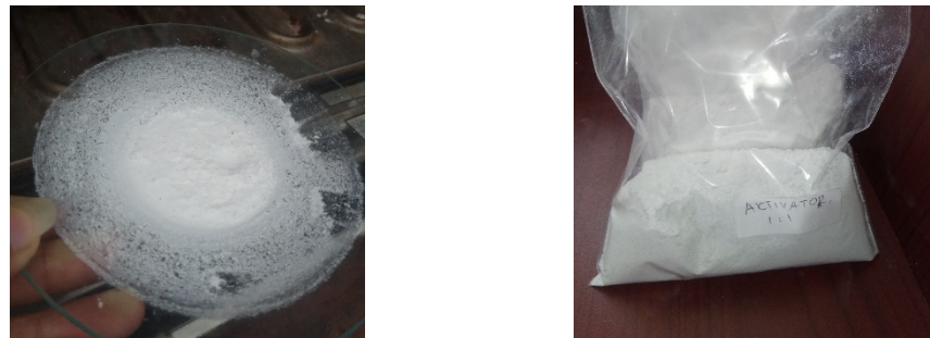
Figure 1. Dry activator synthesized by mixing NaOH and geothermal silica with a ratio of 1:1 (wt./wt.) and then calcining at 400 °C.
