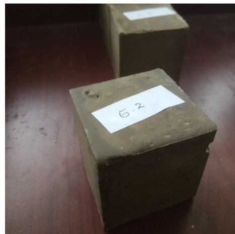
Figure 2. Mortar geopolymer made of coal fly ash and dry activator from silica geothermal sludge.
