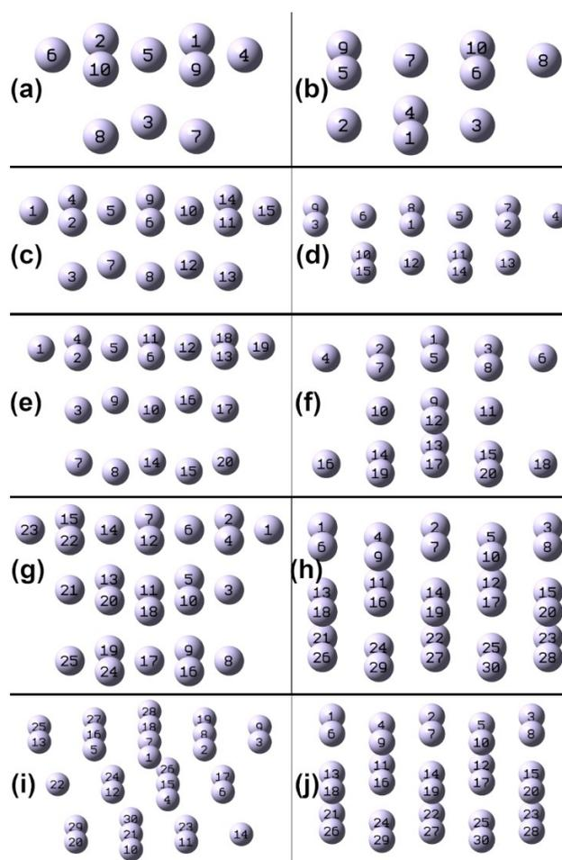
**Figure 1.** Ir<sub>n</sub> clusters modelled, where n = 10, 15, 20, 25, and 30. The left column depicts the (111) surfaces and the right column depicts the (100) surfaces. Atoms are numbered so they can be matched with their respective spin densities in Figure
