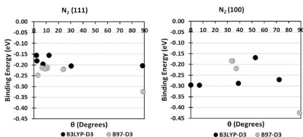
**Figure 5.** Binding energy (based on electronic energies) of N<sub>2</sub> adsorbed on the (111) and (100) surfaces at various angles.  $\theta$  is the angle the N–N bond makes with the catalyst surface.
