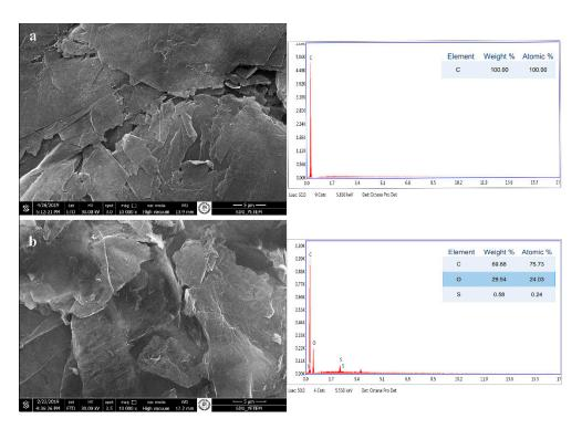
Figure 4. SEM/EDX image of graphite (a) and GO (b).
