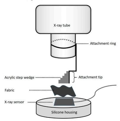
Figure 2. Schematic demonstration of the setup.
