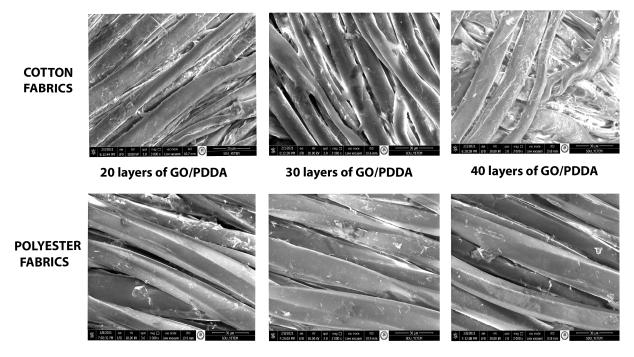
Figure 5. SEM micrographs of GO-multilayer-coated fabrics.
