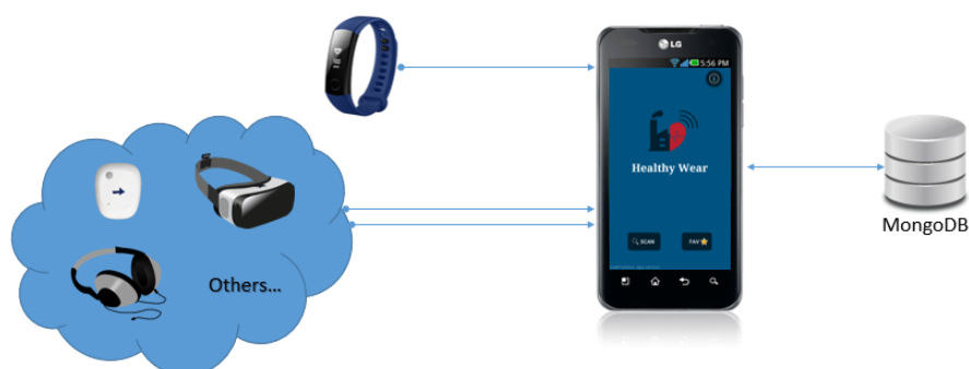
Figure 5. Overview of the applied wearable data flow.
