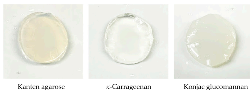
Figure 5. Pictures of biomass hydrogels of Kanten agar, \kappa -carrageenan, and konjac glucomannan.
