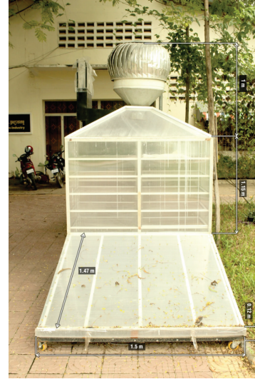
FIGURE 1: The schematic picture of natural convection solar dryer.
