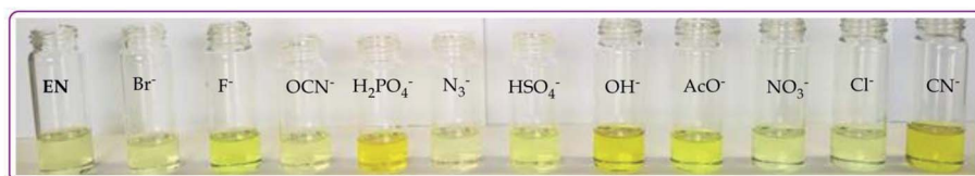
Fig. 5 Observable colorimetric activities of different anions (0.03 M) upon interacting with EN ( 1 \times 10^{-5} M) in DMSO–H 2 O at room temperature.
