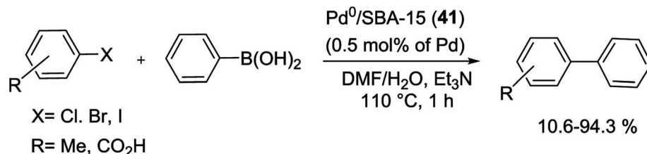
Scheme 53 Pd 0 /SBA-15 (41) catalyzed Suzuki coupling reaction.
