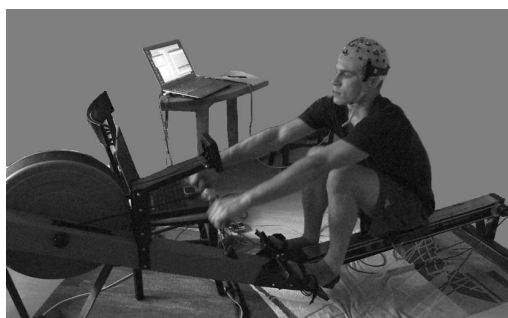
Figure 1. Electroencephalography (EEG) recording during ergometer rowing in pilot Study 3. The Concept II (Model C) indoor rower was used for the pilot studies. The Concept II models are the most frequently used ergometers for training in competitive rowing and performance diagnostics. In the drive phase of the rowing cycle, the rower's pull accelerates an air resistance braked flywheel in the round cage. In the recovery phase, the rower moves in the opposite direction on the sliding seat, preparing for the next pull. A monitor displays the stroke rate, time, distance rowed, power per stroke, mean power, and calories burned. On the chair at the right side in front of the rower is the laptop for stimulus presentation. The laptop on the table recorded the behavioral and EEG data (photo use with participant's permission).
