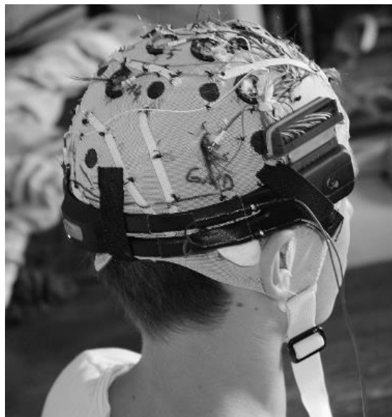
Figure 4. The modified Emotiv system combined with a standard electrode cap. A connector was fixed above the part of the headset containing the amplifier circuits. The two cables connected the headset with the photodiode used for the synchronisation of stimulation and EEG recording at the start and end of each experimental run. During rowing, the cables were removed.
