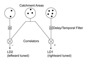
**Figure 2. A modified Reichardt detector.** This forms the basis of the local detectors in the module. Output from LD1 is excitatory and indicates rightwards motion. Output from LD2 is inhibitory and indicates leftwards motion. In this modified detector the central catchment area that samples in the neighbourhood of (x,y) in the first-field is shared between LD1 and LD2 (see text). doi:10.1371/journal.pone.0042995.q002
