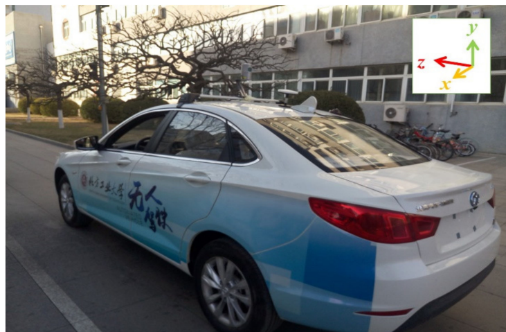
Figure 5. Unmanned vehicle carried with LiDAR sensor.
