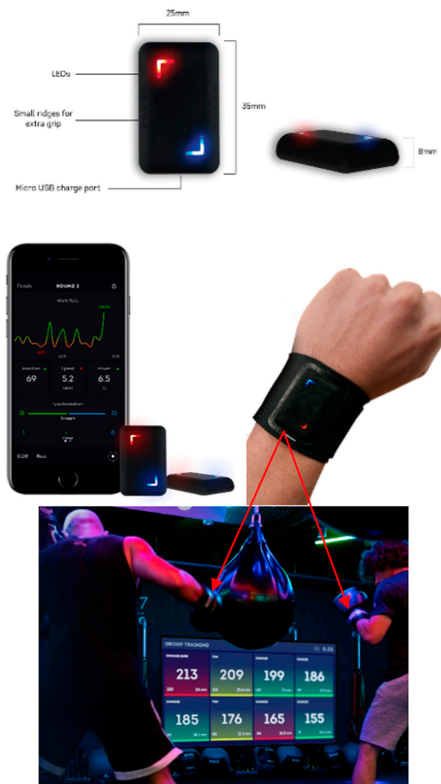
Figure 18. Corner Boxing System: Sensor with dimensions (top), sensor, phone app and wrist attachment (middle), and sample group training session with data from several users compiled and displayed simultaneously (bottom).
