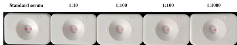
**Figure 13.** Experimental results of RVFT detection limit.
