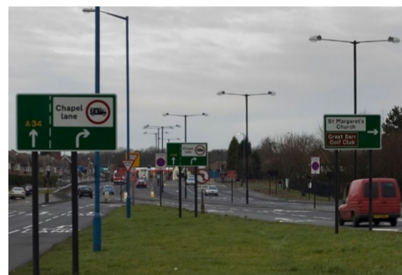
Fig. 3 An example of edge case related to multiple signs. An autonomous system may interpret all visible signs as relevant, even though some relate to a parallel road. "Furniture" by hartlandmartin is licensed with CC BY-NC-SA 2.0
