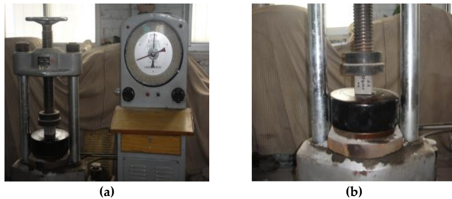
Figure 4. Compressive strength test: (a) compression testing machine; (b) test pieces of loading.
