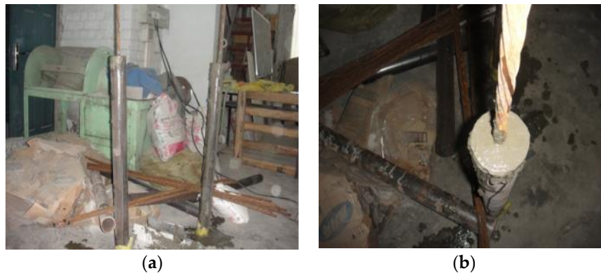
Figure 5. Bond stress test piece: (a) exterior; (b) interior.
